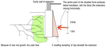
Because of new root growth, the outer face of clay shrinks away seasonally, exhibiting progressive movement as the force from the inner face (beneath the building) prevents closure. Monitoring shows opening in the summer and no movement in the winter. A 'swelling dumpling' of clay beneath the extension exerts lateral pressure against the inner face of the deep trench fill which should have had a compressible fill behind it.
